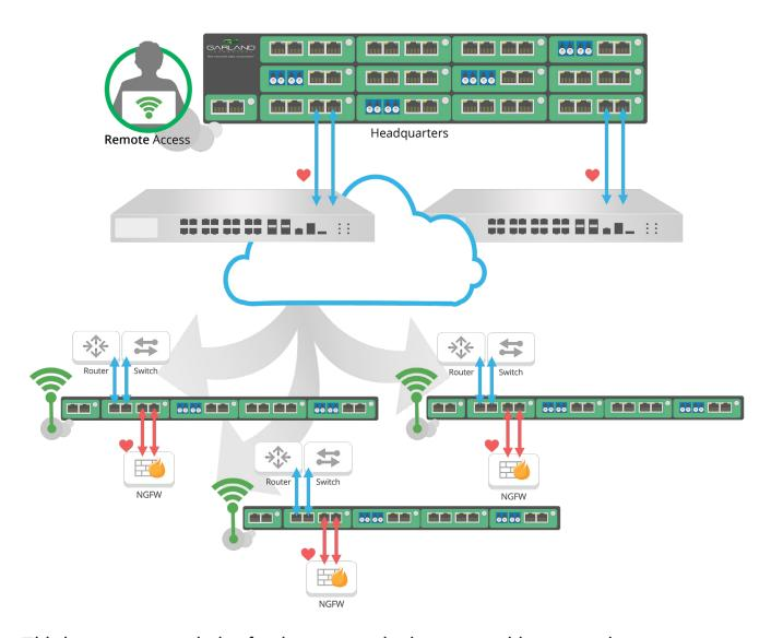
This is a common solution for data center deployments with remote site management (retail, banking, etc.). The data center houses two in-line, active security appliances. The remote sites, connected via the cloud, require their own two in-line, active security appliances.
