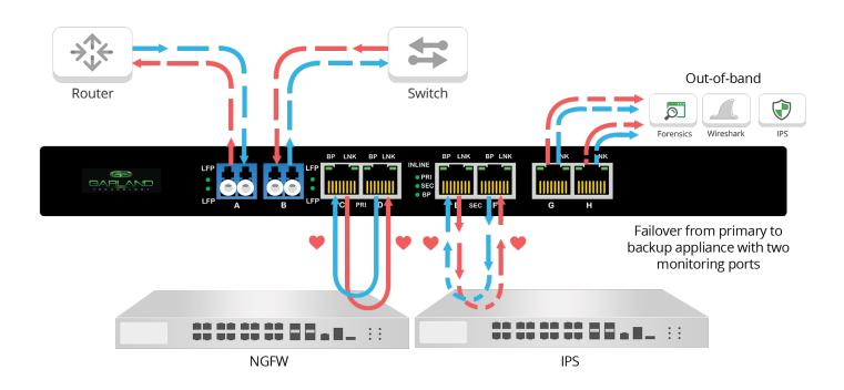
This solution again offers a single bypass TAP that can support two in-line security appliances; however, it is specifically designed for high availability environments.
